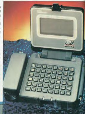
Badger's GT-110 weighs 30 ounces, uses several battery types, has a PC Card Type I slot, is PCcompatible, and satisfies military specifications for temperature, rain, vibration, and other challenging environments.
